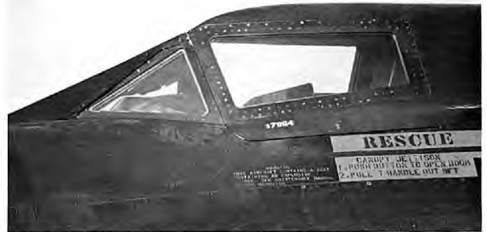
Canopy of 17964. These windows will reach temperatures of up to 400 degrees Fahrenheit in Mach 3 flight, enabling crews to heat the tube food carried on operational missions by holding it against the window for a short period. (Ted Carlson)
