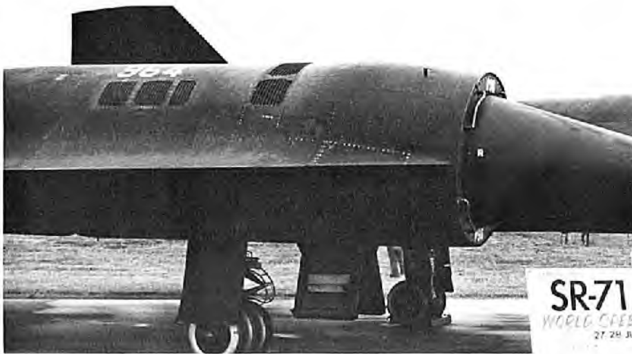
(Left) The secret of the SR-71's ability to maintain high cruise speeds for long periods of time is in the automatically programmed inlets, which provide up to 60% of the thrust above Mach 3. (Charles B. Mayer)
