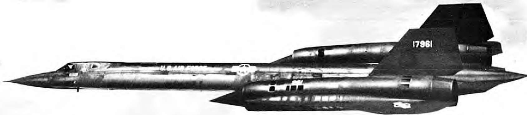
(Above) Actual paint used on the Blackbird has been quoted as being FS 35402 Indigo Blue, but it is as black as any FS black. (Lockheed)
