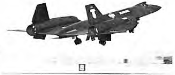
06935 gets away on a test flight. Note that the center ventral fin has begun to unfold as the gear begins its retraction cycle. (Lockheed)
