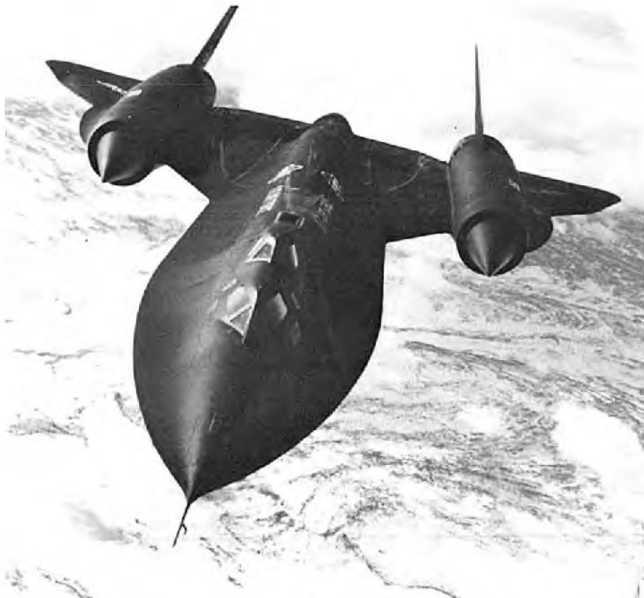
The only currently operational two-pilot Blackbird is SR-71B #17956, seen here about to take on a load of JP-7 from a KC-135Q of 100th ARW. (Author)
