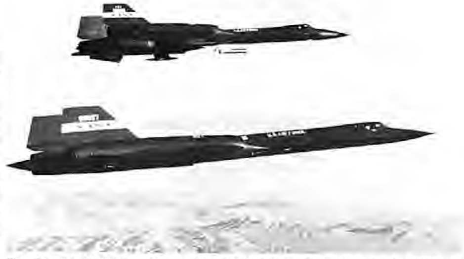
The Second YF-12A, equipped with a Coldwall experiment to study effects of aerodynamic heating on a cylinder cooled with gaseous nitrogen. (Large cylinder under fuselage) It has also been fitted with the camera pods originally installed on 06934 to record missile firings. The SR-71 prototype (sometimes referred to as the YF-12C) is flying chase. During one test flight, these two aircraft experienced nearly simultaneous unstarts. The YF-12 actually lost both engines and had to relight them at lower altitude. (NASA)
