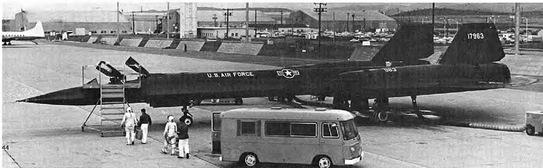
SR-71 Crew about to board at Beale. Prior to installation of a permanent starting system in the SR-71 hangars at Beale, starter carts using twin Buick V-8's with a common drive shaft were needed to provide the starting power for the J-58. (USAF)
