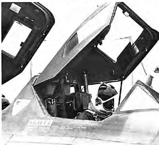
The suit worn by SR-71 crewmen is identical to that now used in the Space Shuttle. It is the principle protection in the event of an ejection at high Mach and altitude, and has been proven in several cases to be effective. (Author)
