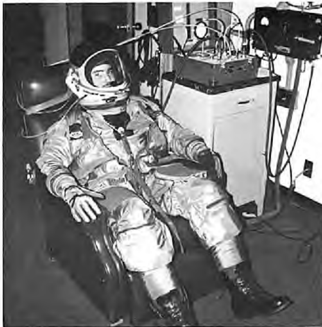
The suit worn by SR-71 crewmen is identical to that now used in the Space Shuttle. It is the principle protection in the event of an ejection at high Mach and altitude, and has been proven in several cases to be effective. (Author)
