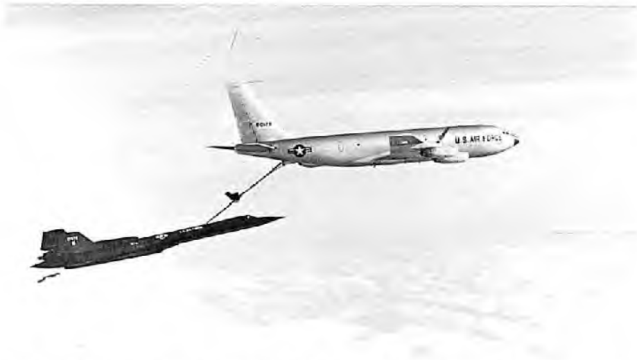
The Rapid Rabbit refuelling from a KC-135Q. Though the JP-7 is kept in separate tanks in the tanker, crew members report that they are able to burn it if necessary in the tanker engines. (USAF)
