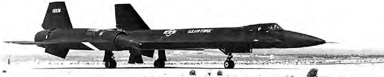
YF-12A #06936 taxis in after a test flight. Note that the drag chute compartment doors are still open. White markings on undersides were to aid in calibration of record-run instrumentation during the record-setting flights of May 1, 1965. (Lockheed)
