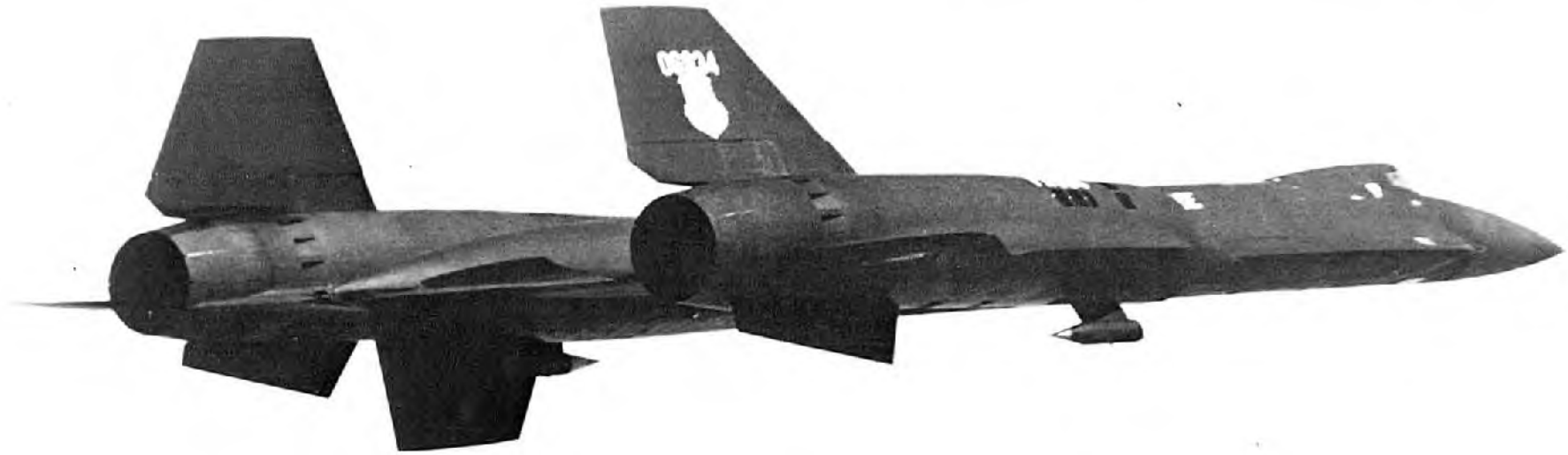
The redesign of the nose shape to accommodate the YF-12A Fire Control System is obvious in this bottom view of the Fighter version of the Blackbird. (John Mallozzi)
