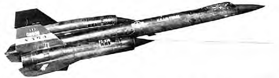
(Above) One of the most startling of NASA discoveries was the fact that, at Mach 3, 50% of the Blackbird's drag was generated by air vented out of the bypass doors. (NASA)
