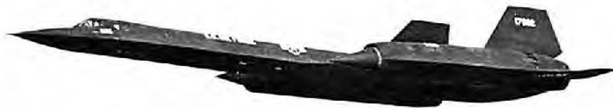
17962 during a fly-by at Beale in July, 1976. Aft by-pass doors are open below about Mach 1.2. (Charles B. Mayer)
