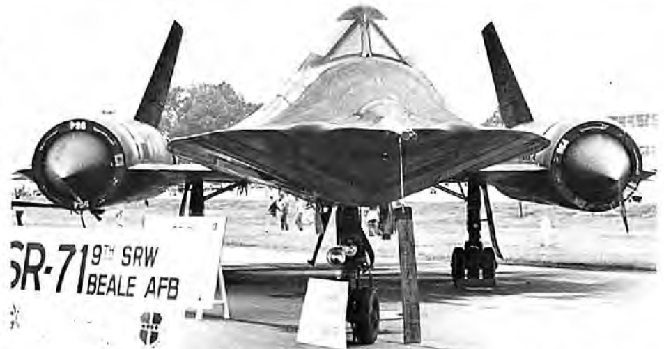
Latest modification to the nose of the SR-71 interrupts the smooth line of the chines with ECM "dents". (C.B. Mayer)
